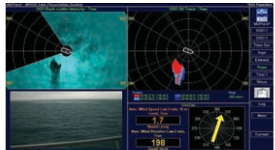
The tactical display of the Miros OSD system presenting a back scatter intensity image and the corresponding Trace image.
