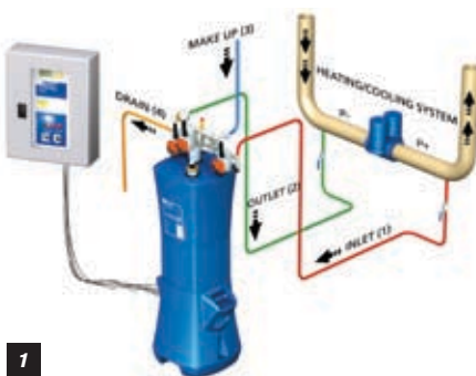
1. Maritime water treatment by EnwaMatic®. Patented worldwide.
