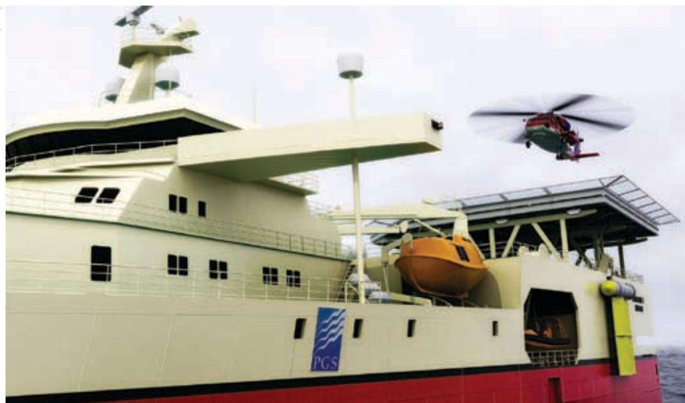
TTS Active Roll is a motion-compensated helideck system that improves helicopter access to moving sea vessels.
